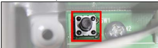
Reset switch at top-left inside corner
